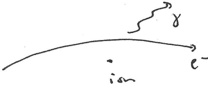
Figure 20: Bremsstrahlung (braking radiation) — an electron decelerates near an ion and emits a photon.
