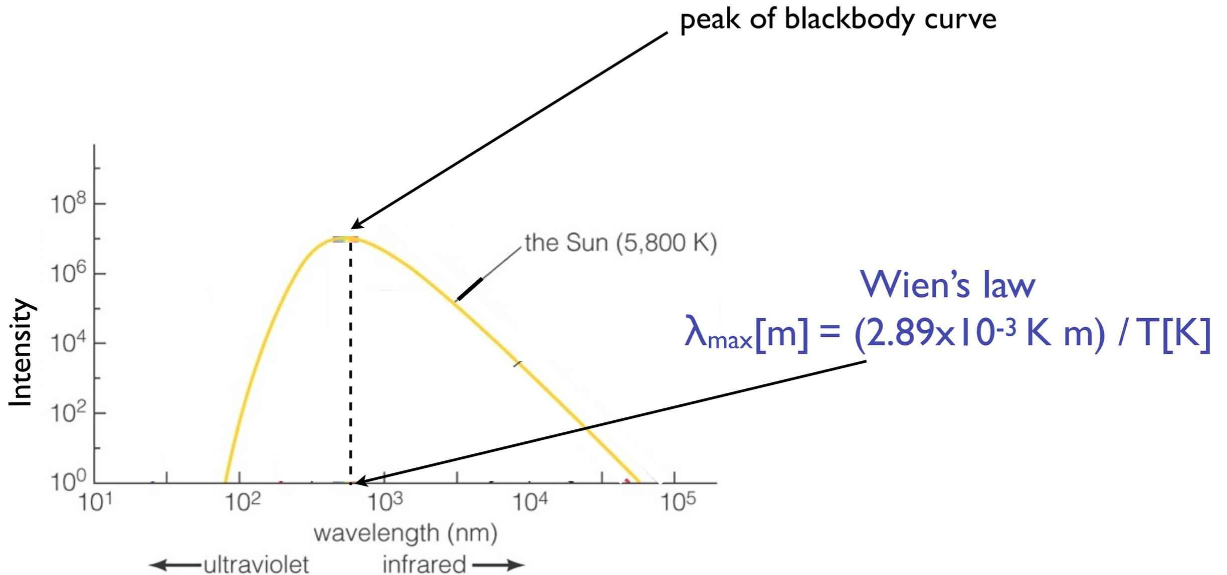
The **WAVELENGTH** that the **PEAK** of the blackbody curve occurs at tells us about the object's **TEMPERATURE** and **COLOR**.
