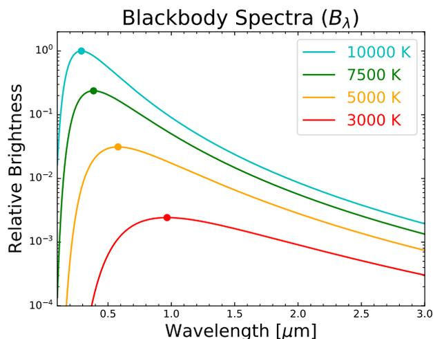
Figure 3: Blackbody spectra  $B_{\lambda}(T)$  for a range of temperatures  $T$ . The temperatures used here correspond roughly to the range of  $T_{\text{eff}}$  spanned by the stars shown in Fig. 4. The circular points indicate Wien peak of each blackbody.
