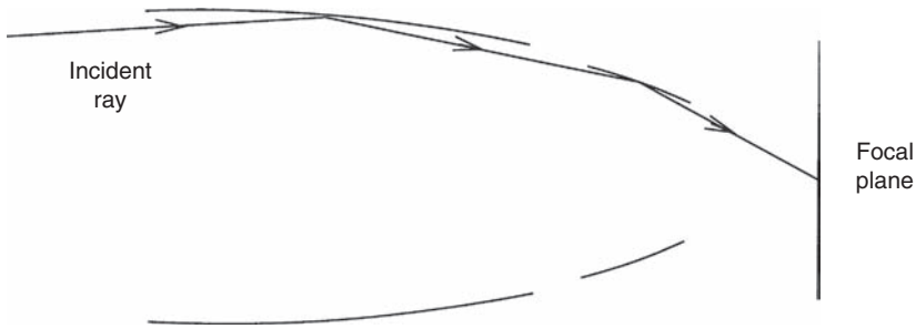
Fig. 1.6 A schematic representation of the optics of an X-ray telescope, in which X-rays are focused by two successive reflections at grazing incidence.
